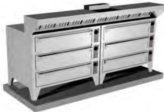
2. An eyebrow hood that will extend the full length of the oven with the inside edge of the hood overhang of the oven door opening(s) by at least 36-inches. Use the formula  $Q=50A$  to calculate minimum hood exhaust volume.
